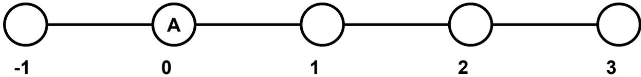
**Figure 1.** Diagrammatic representation of aggregate transportation distance from single production site (A) to supply five projects (circles). Numerical scale indicated in miles (Adapted from Berek, 2005).
