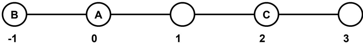
**Figure 2.** Diagrammatic representation of aggregate transportation distance from two production sites (A and, B or C) to supply five projects (circles). Numerical scale indicated in miles (Adapted from Berek, 2005).
