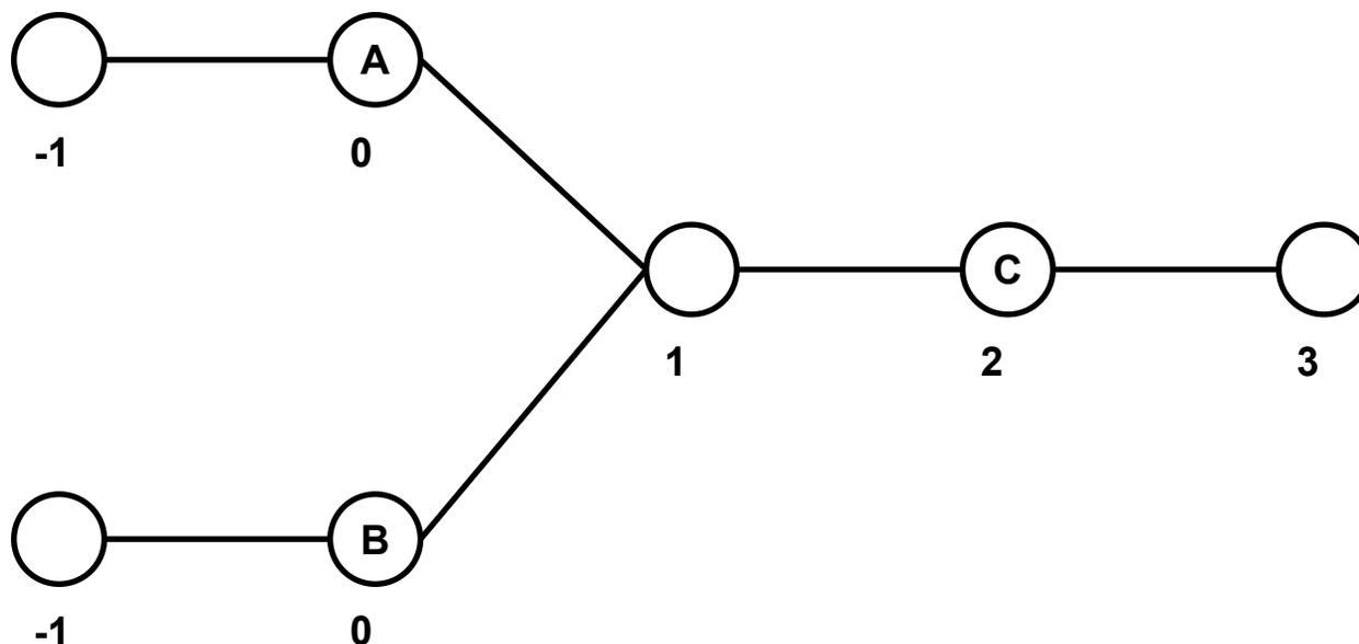
**Figure 3.** Diagrammatic representation of aggregate transportation distance from two production sites (A and, B or C) to supply five projects (circles). Numerical scale indicated in miles (Adapted from Bereck, 2005).
